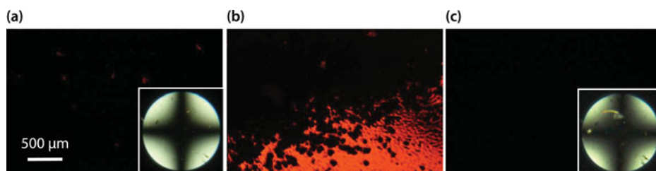
Figure 5. POM images under crossed polarizers of ZLI-4792/D-6A5 mixture (99/1, wt/wt) (a) before, (b) just after, and (c) 2 minutes after the UV irradiation
